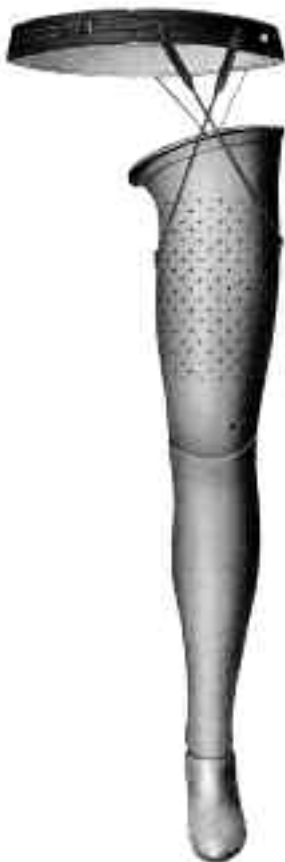
Figure 37. This light-metal leg, circa 1936, was used in cases of amputation above the knee. The Hanger company was the first to form the shin of the leg in a one-piece seamless pressing drawn from a flat sheet, resulting in a much lighter and stronger leg.
