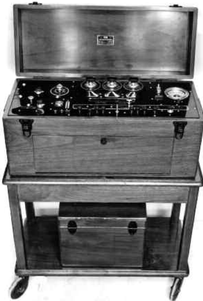
Figure 43. This electrocardiograph (ECG), manufactured by General Electric, includes a rolling stand, battery case, and amplifier unit. The ECG has become one of the most widely used diagnostic tools.
