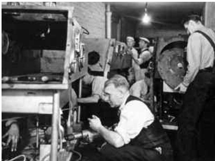
Figure 29. Hospital staff constructing steel tank respirators in the basement of Toronto’s Hospital for Sick Children in 1937. These “homemade” iron lungs were used successfully in many cases, but were soon replaced by American commercial models.
