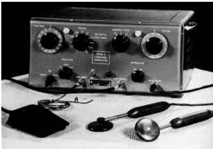
Figure 44. Jack Hopps and his co-workers at the National Research Council built this external pacemaker in 1951. It was a combined stimulator-defibrillator, with a foot pedal to trip the single 200-volt defibrillating shock. (W. G. Bigelow, Cold Hearts: The Story of Hypothermia and the Pacemaker in Heart Surgery [Toronto: McClelland & Stewart, 1984], 108)
